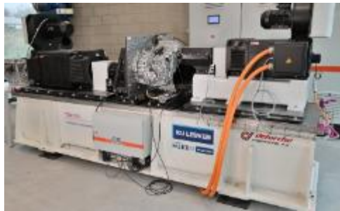
FIGURE 4: GEARBOX AND BEARINGS TEST RIG
