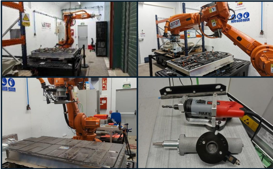
FIGURE 13: MOVABLE IRB6620 ROBOT ARM WITH SOME OF THE AVAILABLE TOOLS
