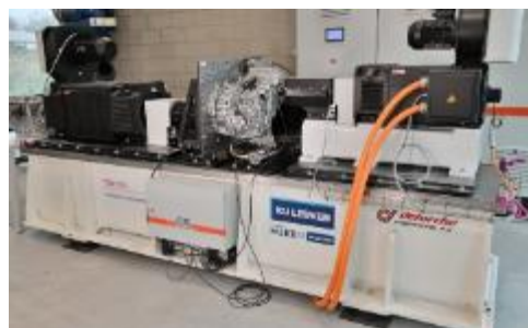
FIGURE 4: GEARBOX AND BEARINGS TEST RIG
