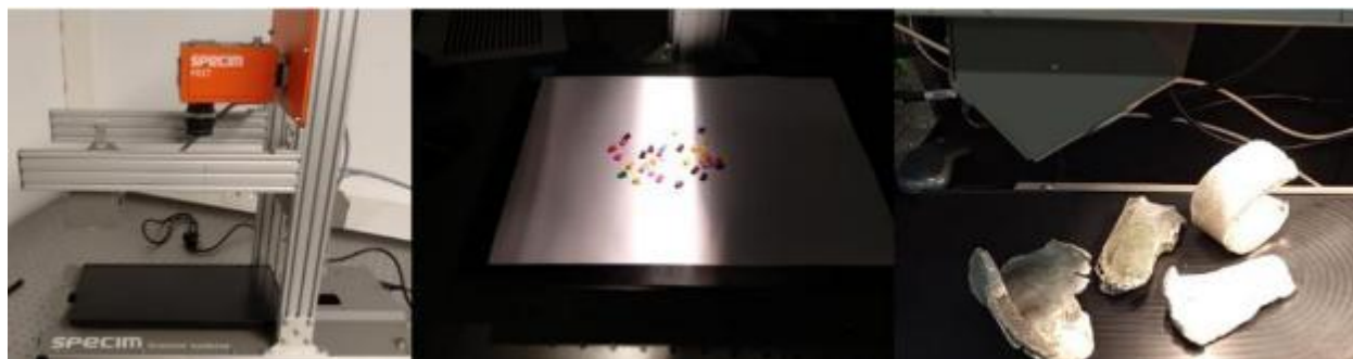
FIGURE 16: FROM LEFT TO RIGHT: HYPERSPECTRAL CAMERA, CAPTURE OF IMAGE OF POLYMERIC SAMPLES AND METALLIC SAMPLES.
