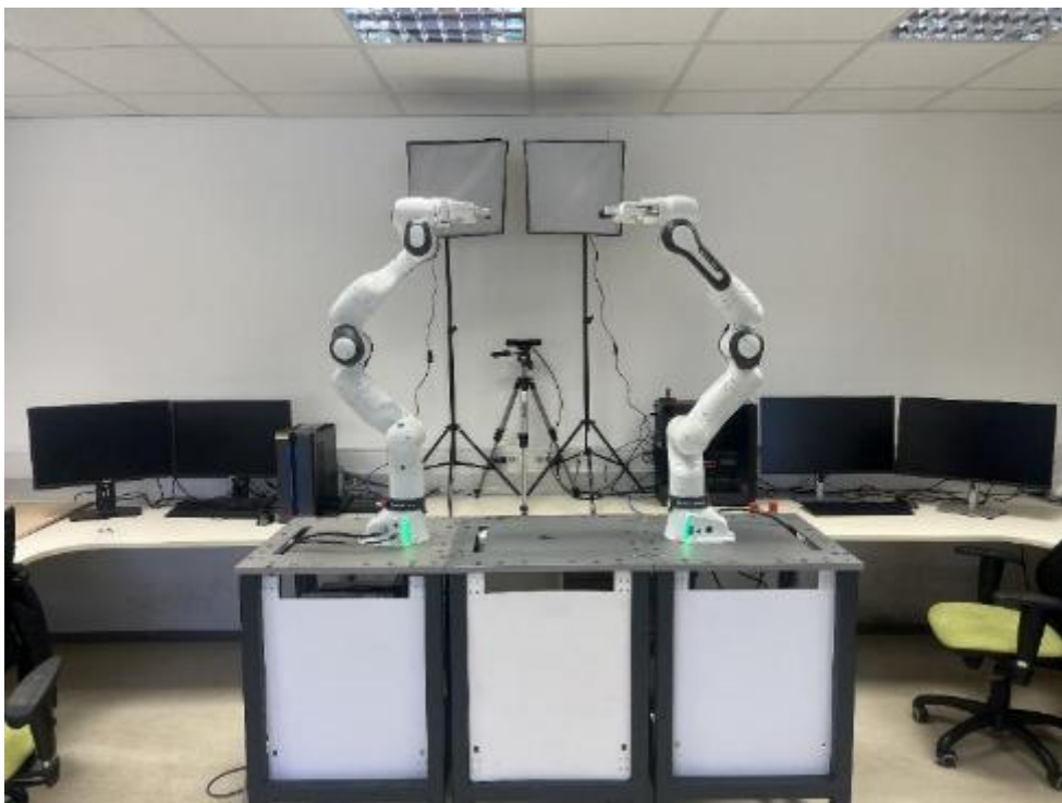
FIGURE 12: MODULAR ROBOTIC CELL WITH TWO FRANKA EMIKA FR3 COLLABORATIVE ROBOTS
